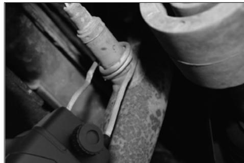
2. Bend the coil in the way that looks like the drawing on the right and relevant to the size of the dent.
